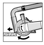
Switch on the machine and place the front part of the cutting guide on the workpiece. Slide the machine with moderate feed, adapted to the material to be worked.
